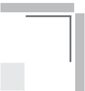
Open exterior corner with hidden profile.
