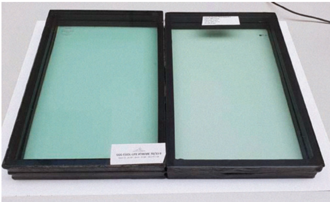
Solar control glass Xtreme 70/33 with inner glass Planitherm XN left and ECLAZ right.
