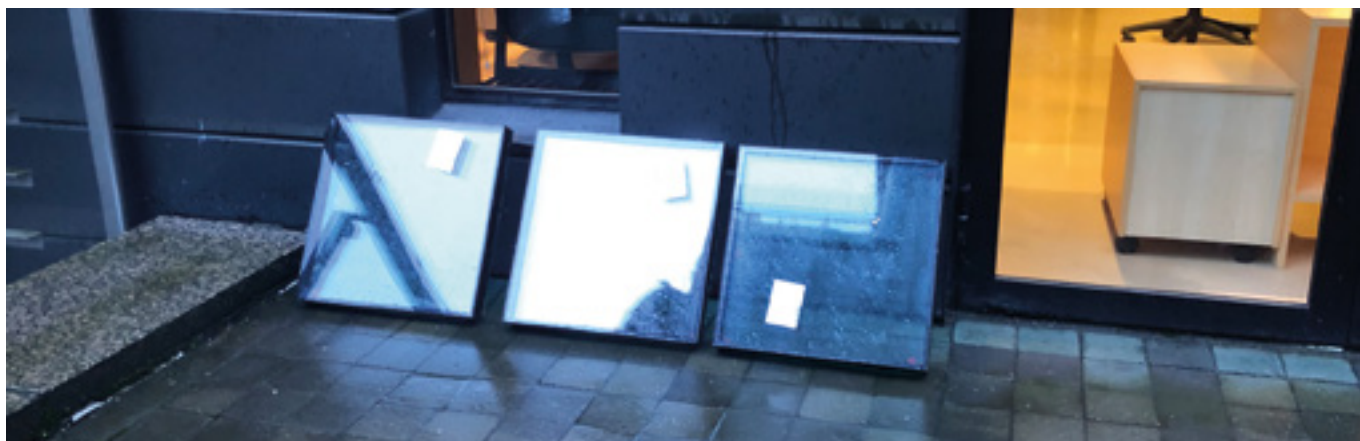
Outer pane left to right: Xtreme 70/33 Diamant Float Xtreme 70/33 Diamant / Planiclear laminated
